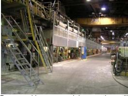
Paper machine press and dryer sections still installed in Canada.
